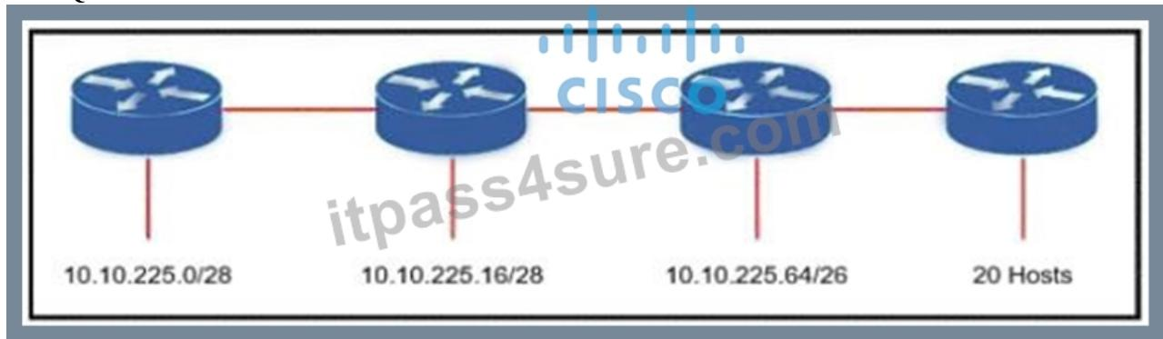
Refer to the exhibit. An engineer must add a subnet for a new office that will add 20 users to the network. Which IPv4 network and subnet mask combination does the engineer assign to minimize wasting addresses?
