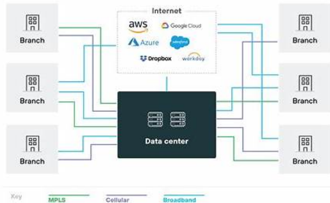
SD-WAN architecture with multiple branch sites and cloud applications
