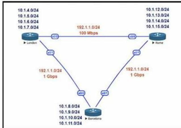
This network is running OSPF as the routing protocol. The internal networks are being advertised in OSPF. London and Rome are using the direct link to reach each other although the transfer rates are better via Barcelona. Which OSPF design change allows OSPF to calculate the proper costs?
