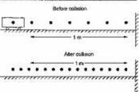
In the laboratory, a 0.5-kg cart collides with a fixed wall, as shown in the preceding diagram. The collision is recorded with a video camera that takes 20 frames per second. A student analyzes the video, placing a dot at the center of mass of the cart in each frame. The analysis is shown above.
