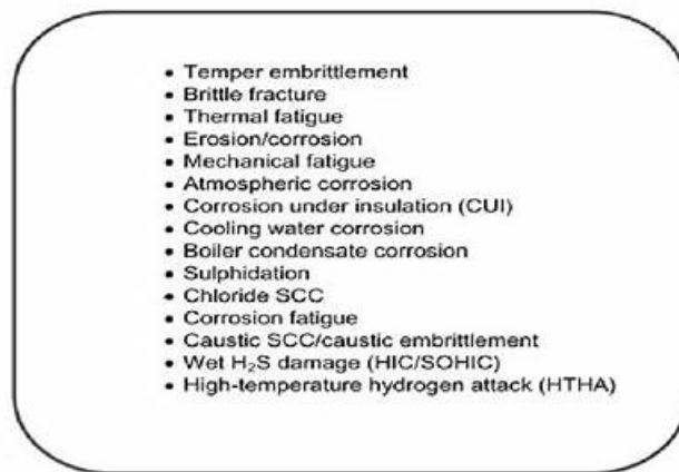
Figure 7.1 The 15 damage mechanisms from API 571 in the API 510 exam syllabus
