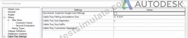
An electrical designer models a cable tray in a project and decides to check the box (or Use Annot. Scale tor Single Line Fittings and change the Cable Tray Fitting Annotation Size to 1/8" (3 mm).
