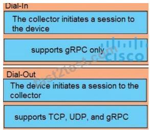
In a dial-in mode, the destination initiates a session to the router and subscribes to data to be streamed. Dialin mode is supported over gRPC in only 64-bit platforms In a dial-out mode, the router initiates a session to the destinations based on the subscription. All 64-bit IOS XR platforms (except for NCS 6000 series routers) support gRPC and TCP protocols. All 32-bit IOS XR platforms support only TCP.
