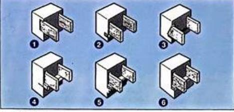
Figure 5.13 Sketches showing various arrangements for supporting floor joists: (1) joist with square end in pocket; (2) joist carried on wooden wall plate; (3) joist with splayed end in pocket; (4) joist carried on wooden wall plate carried on bracket; (5) joist carried on wooden wall plate on corbelled brickwork; (6) joist carried on wooden wall plate on a ledge formed by reducing the thickness of the wall.
