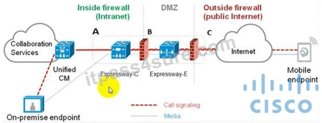
Refer to the exhibit. When making a call to a Mobile and Remote Access client, what are the combinations of protocol on each of the different sections A-B-C?
